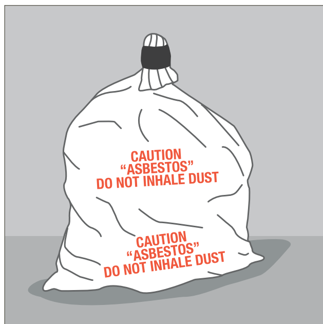
Figure 10: An asbestos waste bag with appropriate warnings.
