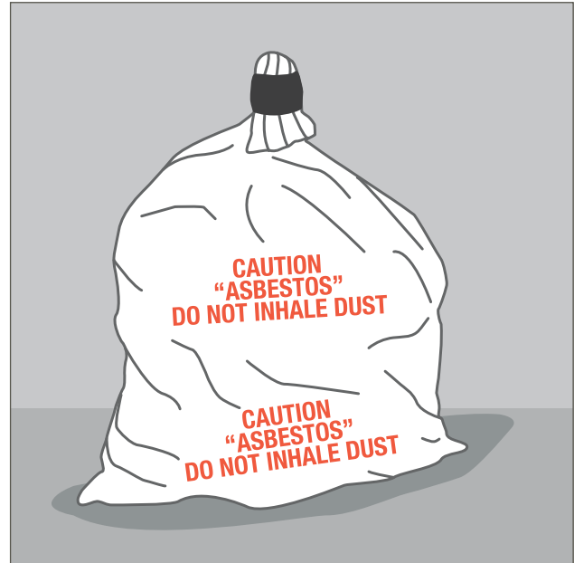
Figure 9: An asbestos waste bag with appropriate warnings.
